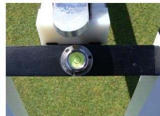
3. When set level, moving the ball release mechanism to the top of the 'Greenstester' provides the same release velocity as the Stimpmeter. The 'Greenstester' can thus be used to measure green speed.
