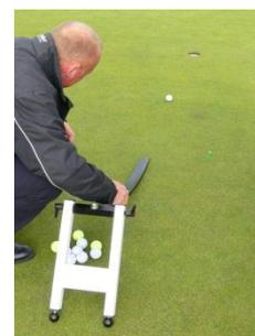
8. To test for a length of putt above green speed, e.g. a 10' putt on a green running at a speed of 9', set the ball release mechanism to the top of the 'Greenstester', adjust the stand to a more vertical position and adjust the feet to raise the 'Greenstester'.
