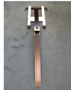
2. Set up the 'Greenstester' so that its feet are not extended and the level bubble is centred.
