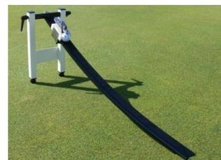
4. To test for any length of putt below green speed, e.g. a 3' putt on a green running at a speed of 9', move the ball release mechanism down the 'Greenstester', fit a ball\* into the release mechanism and roll the ball to assess where the mechanism should be fixed.
