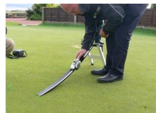
5. On the putting surface to be tested, carry out trial runs to line up the 'Greenstester' to the hole position of the day from the distance to be assessed. Balls missing the hole should only run on for one full rotation of the golf ball, i.e. 5¼ inches (13.4 cm) beyond the front edge of the hole.
